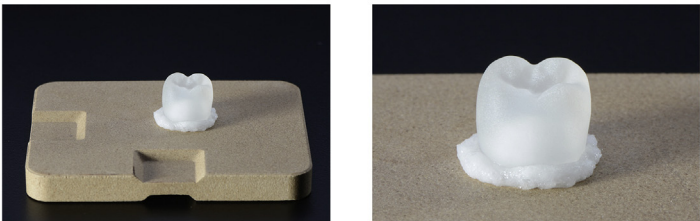
Fig. 1 – Support trays systems used for the crystallization firing of the different groups in this study. Samples of groups 1–3 were placed directly in contact with the firing pin. The lumen of the crowns of group 5 was completely filled with the firing paste, whereas samples in group 4 were placed over the fibrous pad, without any internal filling.
